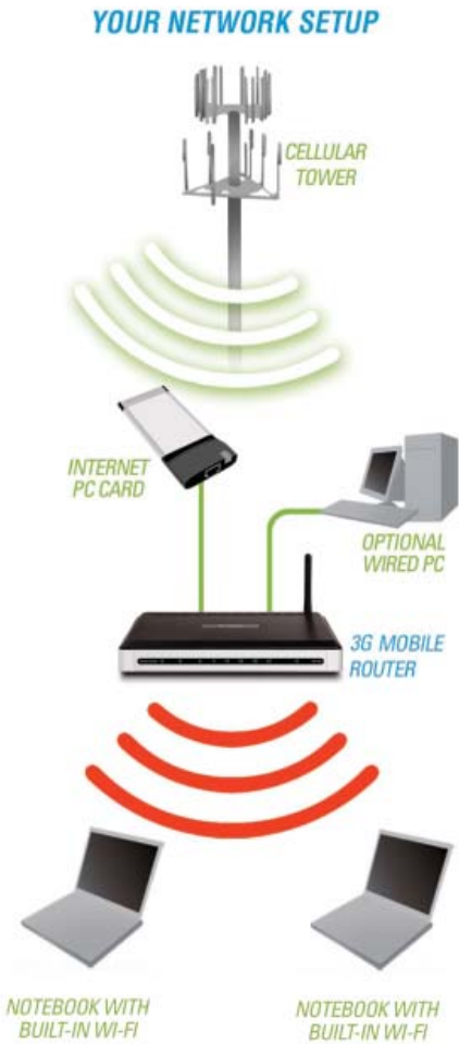
3G Mobile Network Setup: Transform a 3G cellular signal into Wi-Fi for shared network and Internet connectivity.
